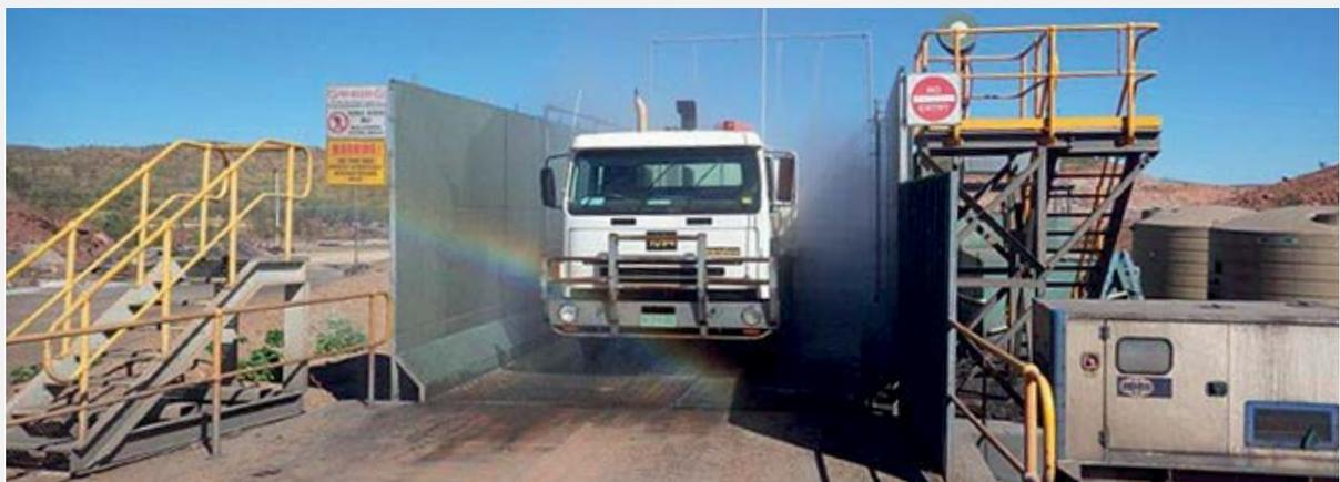
A truck washing station is used at Century to remove hazardous lead dust from vehicles.
